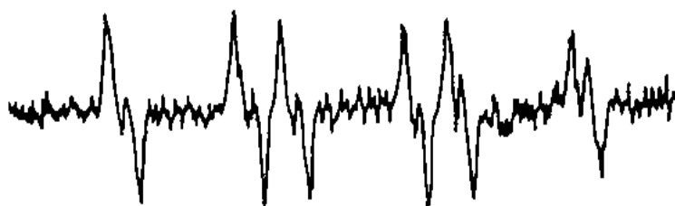
(C) ESR spectrum of DMPO-OOR due to \cdot \text{OOR}
