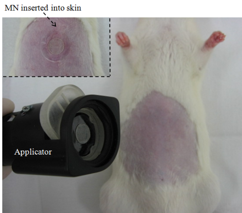
Fig. 23. Sumatriptan succinate-loaded mirroneedle array (MN) was applied to the shaved rat skin with an applicator in the in vivo absorption study.
